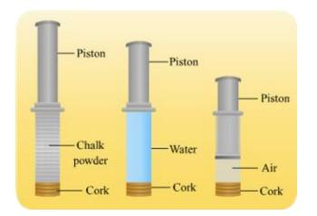
**Result:** The force required to push the pistons of syringes containing chalk powder and water will be greater than that required to push the piston of the syringe containing air.
